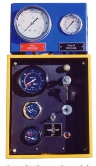
Centralized control panel for engine, high pressure pump, and FRAC-PACKER $^{TM}$ .
